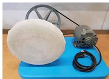
Richardson Buffer – ½ hp 120 vac motor. 12-inch leather buffing disc. $345.00
