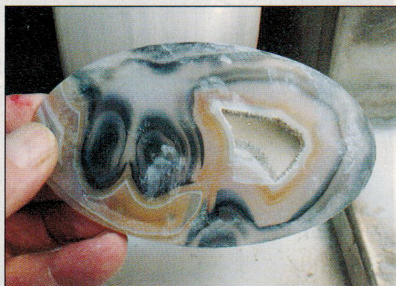
Dry sand the surface with a worn 60 grit silicon carbide belt, checking for flat spots between the first (left) and second passes.
