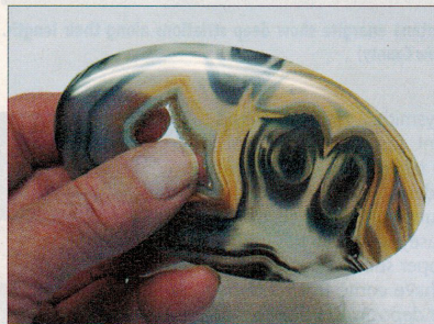
Check for flat spots using the fluorescent light (left). These must be corrected via the wet 100 grit sanding step.
