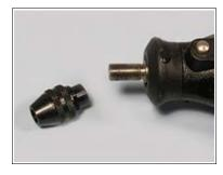
A simple and inexpensive (\$12) adjustable chuck solves all of this. It's available in most large local hardware stores or model-making outlets. Tightening the chuck is done easily by hand to any size shaft. No key is required.
