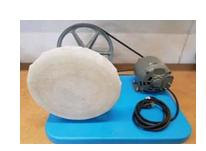
Richardson Buffer –  $\frac{1}{2}$  hp 120 vac motor. 12-inch leather buffing disc. \$345.00
