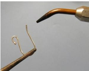
Then it occurred to me - I could melt the wire smooth. One quick touch in the flame of the propane/oxygen Little Torch does the trick - not enough to form a bead on the wire but just enough to round off the tip. I find it's worth practicing the maneuver a couple times on some scrap wire before trying it on completed earrings.
