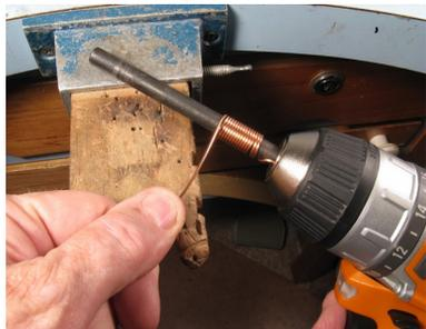
To wind a coil, just bend a right angle on the end of the wire about a half inch long and insert this into the screw gun chuck. Then wind slowly, keeping a tight coil. I like to
