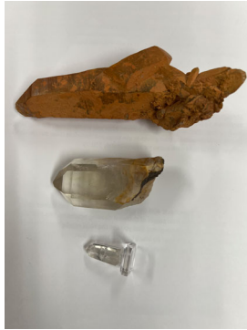
Different stages of cleaned Quartz Crystals from uncleaned to partially cleaned to fully cleaned. Presented by: Thea Stender
